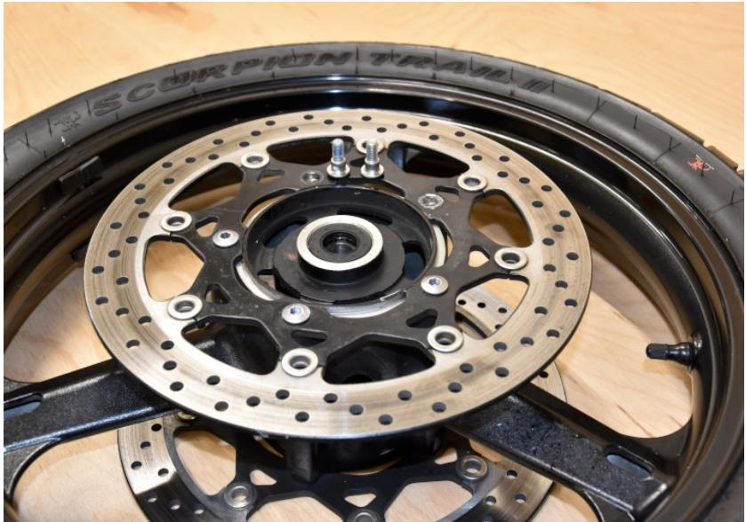
Clean the bolts (remove the threadlocker) and clean that part of the brake disc which will be in contact with the ARA disc.
