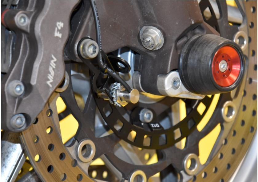
Splice the ARA Green wire to the Brown wire of the speed sensor connector.
