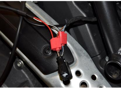
Splice the ARA White wire to the Gray/Green wire at the vertical coil connector.
