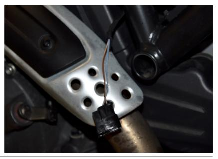
Splice the ARA Red wire to the Brown/White wire at the horizontal coil connector.
