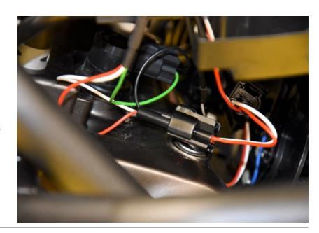
Connect the ARA Black wire terminal to the battery negative terminal.
