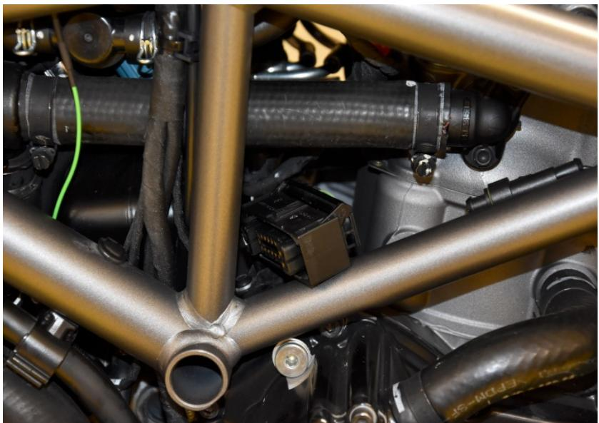
Splice the ARA Green wire to the Blue wire of the ABS connector.(Pin #14)
