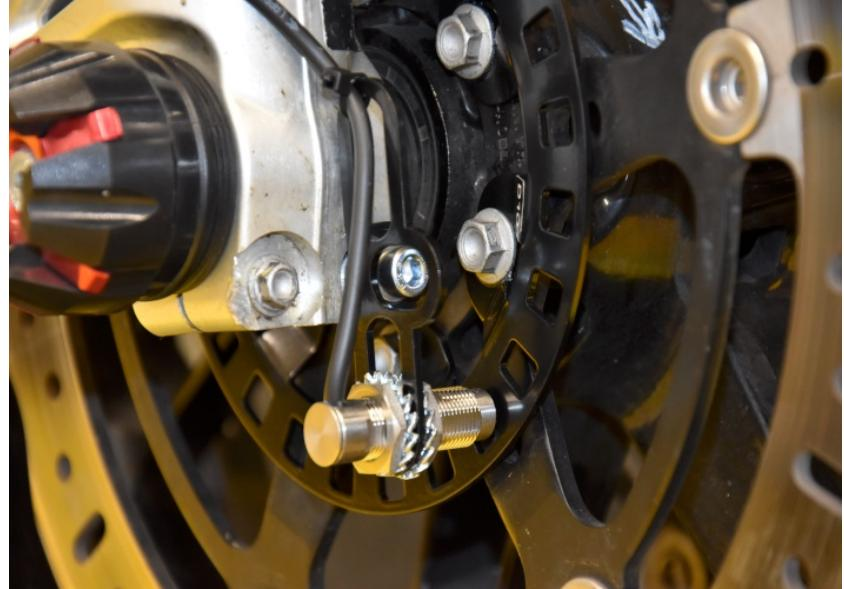
Drill a thread for the rear wheel speed sensor.
