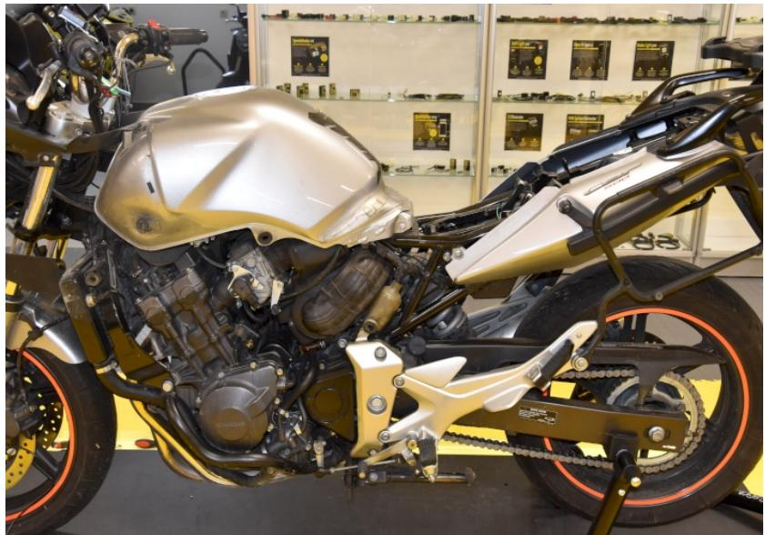
Locate the ignition coil connectors on the right side under the fuel tank.
