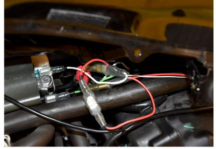
Connect the ARA White wire in-line with the Yellow/Blue wire of the other ignition coil.
