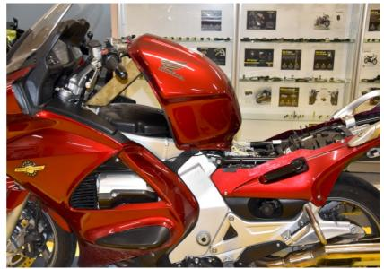
Locate the ignition coil connectors on the left side under the side fairing.
