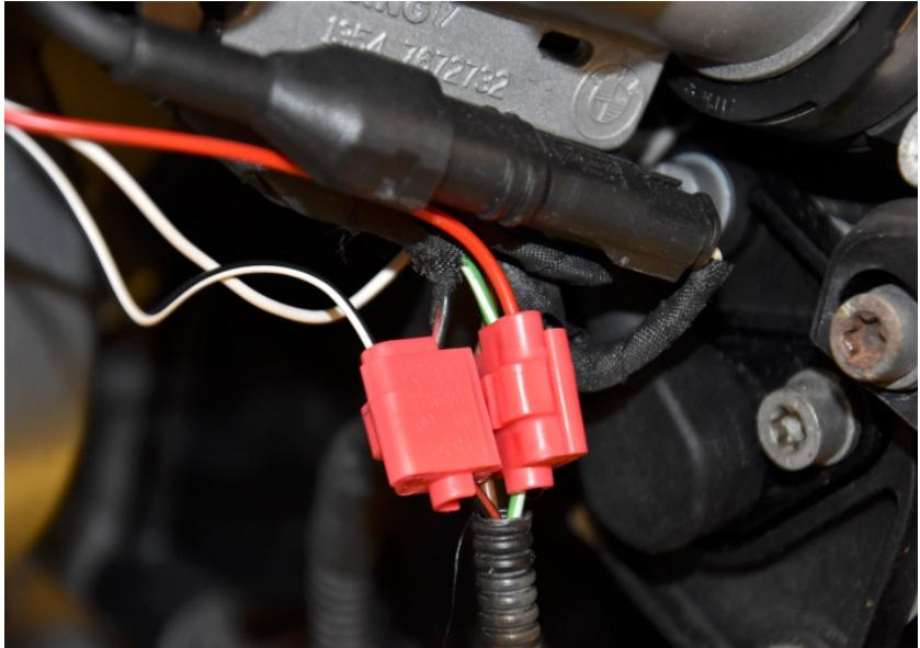
Connect the ARA White wire to the Black/Yellow wire of the auxiliary ignition coil.
