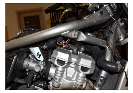
Connect the ARA Black wire terminal to the battery negative terminal.
