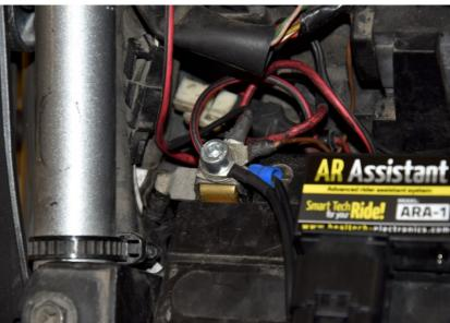
Locate the 10-pole multi connector under the fuel tank.
