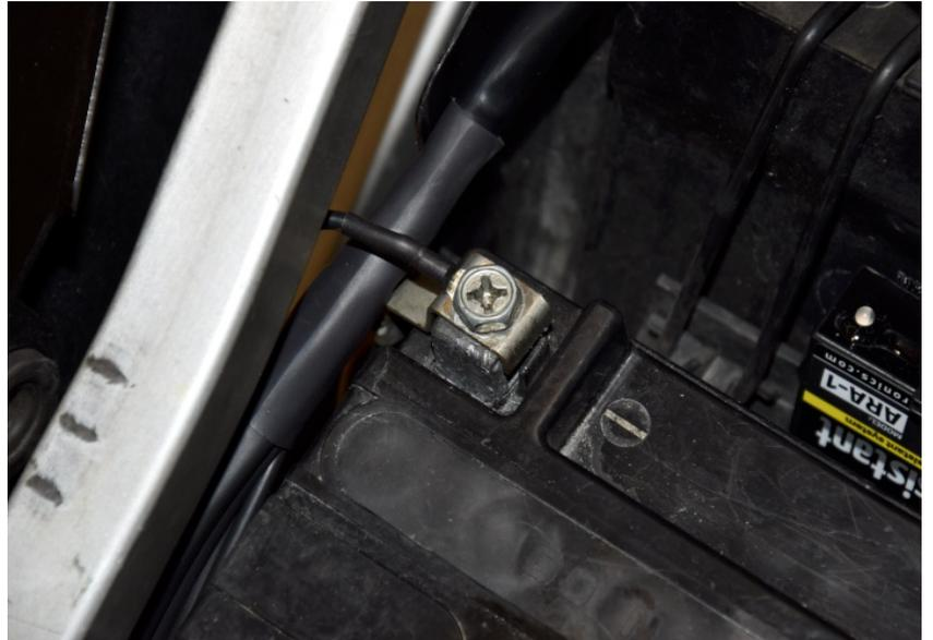
Mount the supplied disk and wheel speed sensor at the front wheel (left side).
