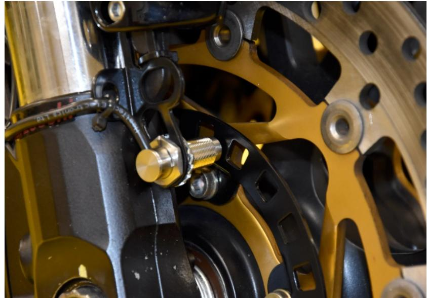
Splice the ARA Green wire to the Brown/Black wire of the speed sensor connector.
