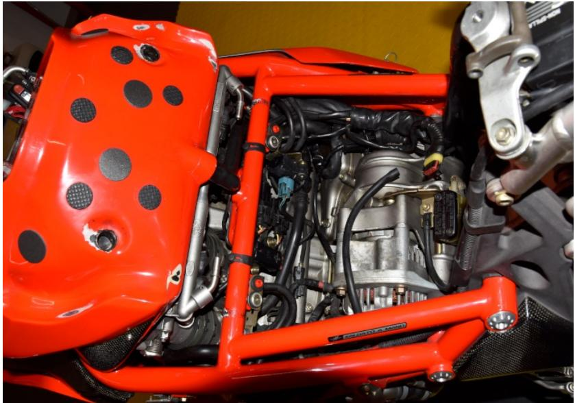
Plug the ARA connectors in-line with the ignition coil connectors.
