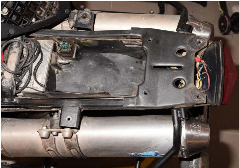
Locate the rear light assembly connector.
