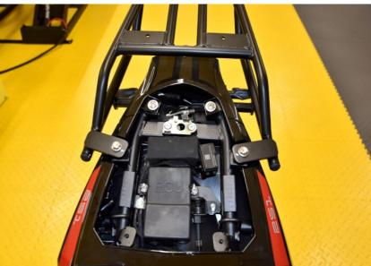
Locate the transparent 3-pole rear light assembly connector in a dust boot.
