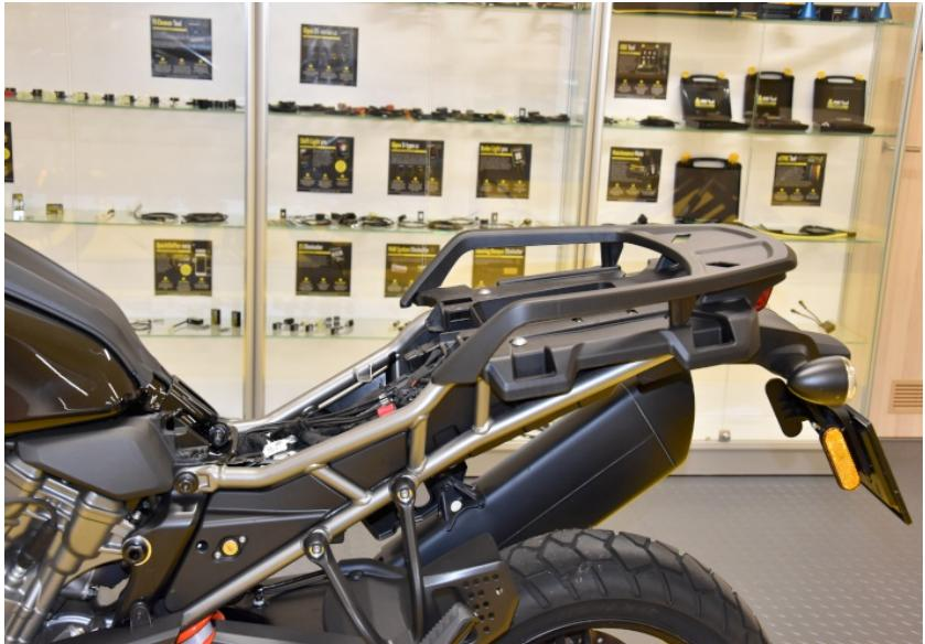
Locate the black 4-pole rear light assembly connector.
