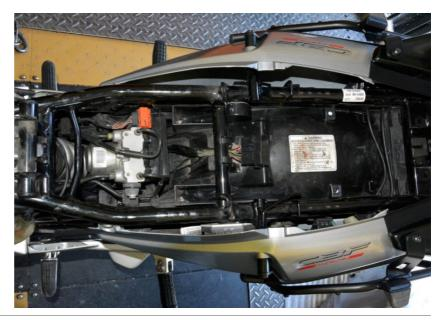
Locate the rear light connector under rear fairing on the left side.
