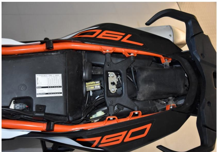
Locate the white 4-pole rear light assembly connector.
