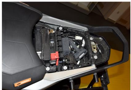
Locate the rear light connector below the passenger seat.
