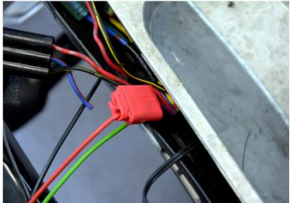
Connect the BLP Green wire to Blue/Red wire end, which goes to the rear light connector.
