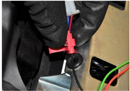
Depress the blade (u-contact) fully with pliers.
