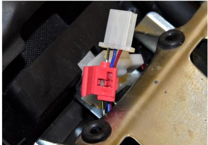
Insert the BLP Black wire completely into the red wire tap.
