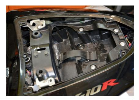
Locate the rear light connector under the passenger seat near the rear light.
