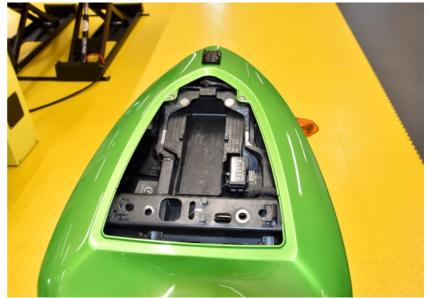
Locate the rear light assembly connector.
