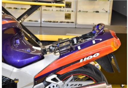
Locate the transparent 3-pole rear light assembly connector.
