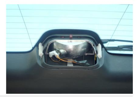
Cut the Orange wire or disconnect the terminal.
