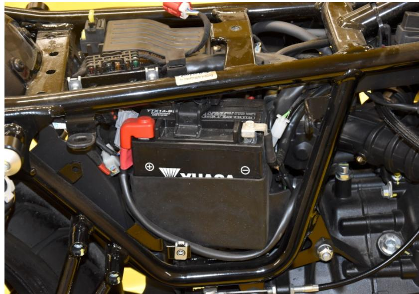
Locate the transparent 6-pole rear light assembly connector.
