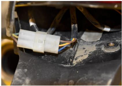
Cut the Yellow/Orange wire of the rear light assembly connector.
