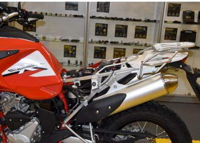
Locate the rear light assembly connector. (White, 8-pole connector on the left side)
