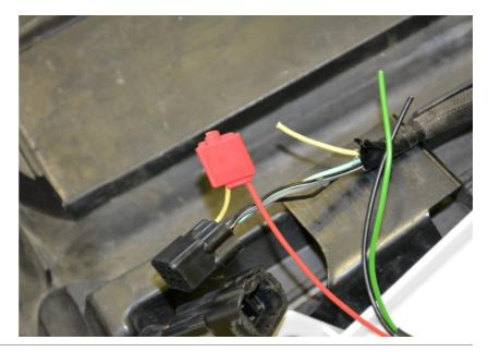
Connect the BLP Green wire to the Yellow wire end, which goes to the rear light assembly.
