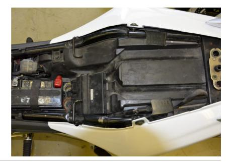
Locate the rear light connector under the seat on the left side.
