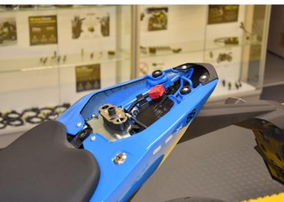
Locate the white 3-pole rear light assembly connector.
