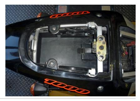
Locate the rear light connector under the passanger seat near the rear light.
