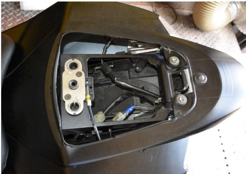
Locate the rear light connector at the backside of the rear light.
