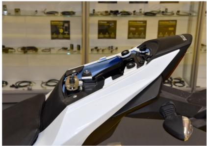
Locate the rear light assembly connector.
