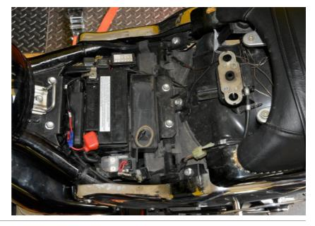
Locate the rear light connector under the main seat.
