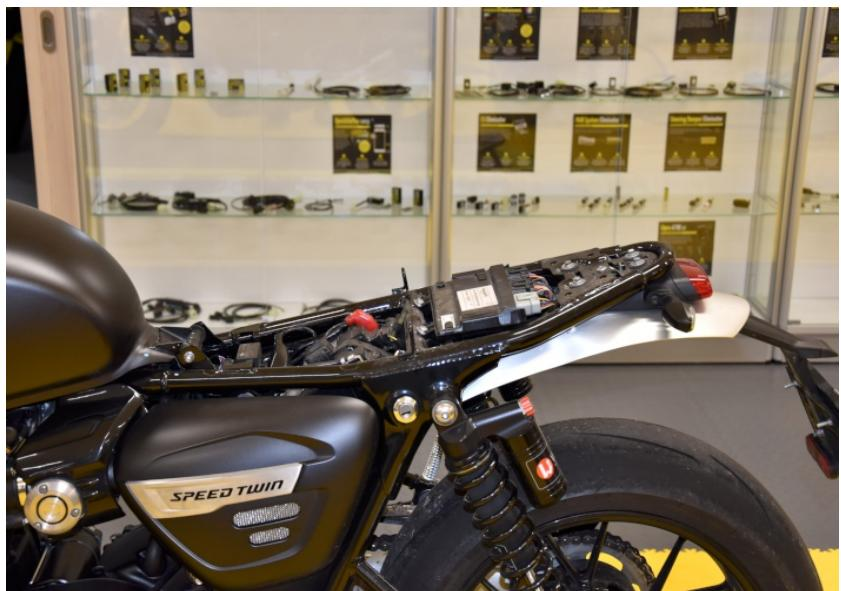
Locate the white 8-pole rear light assembly connector.
