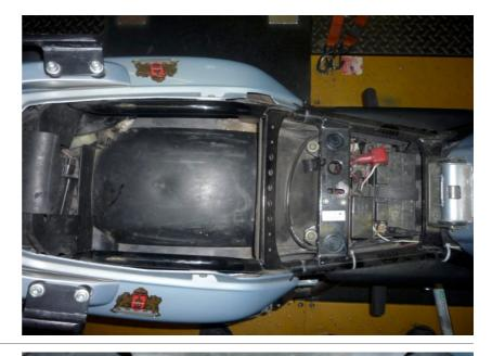
Locate the rear light connector under passanger seat near rear light.
