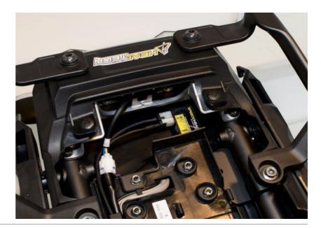
Locate the rear light assembly connector under the passanger seat.
