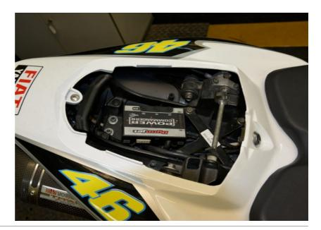
Locate the rear light connector between passanger and main seat.
