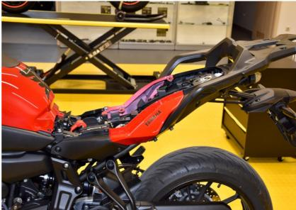
Locate the rear light assembly connector.
