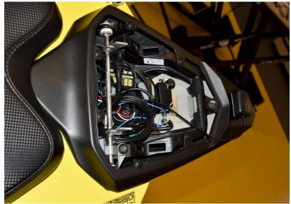
Locate the rear light assembly connector.
