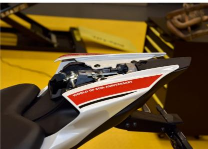
Locate the rear light assembly connector.
