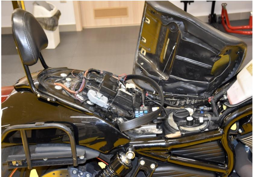
Cut the Black wire of the rear light assembly connector.
