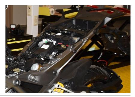
Locate the rear light assembly connector.
