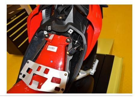
Locate the rear light assembly connector.
