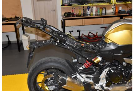
Locate the rear light assembly connector.
