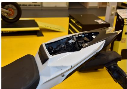
Locate the Black 2-pole rear light assembly connector.
