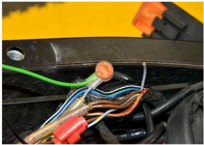
Connect the BLP Red wire to the Grey/Red wire end, which goes to the bike's main wiring harness.
