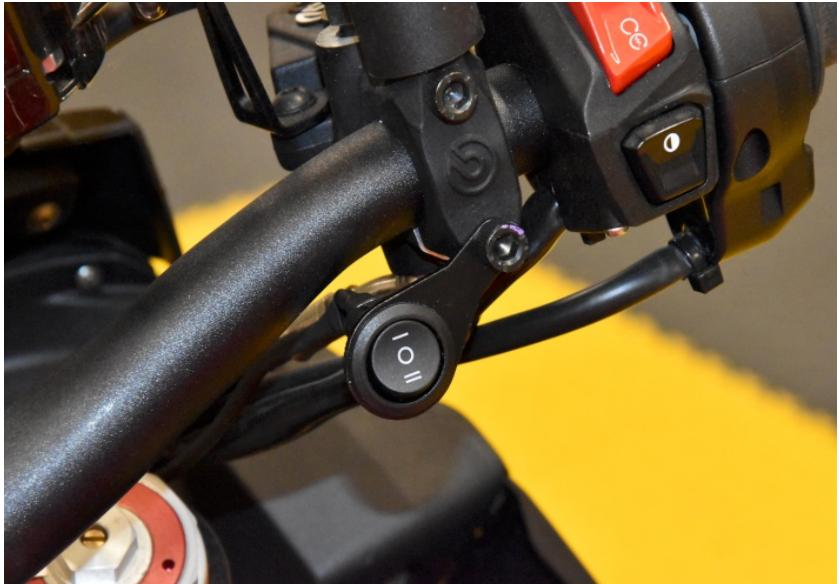
Typical position of the Switchable Exhaust Servo Eliminator module.
