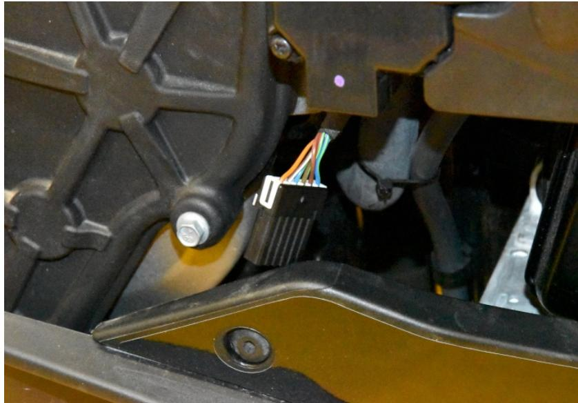
Plug the ESE-SW connectors in-line with the exhaust servo motor connectors.
