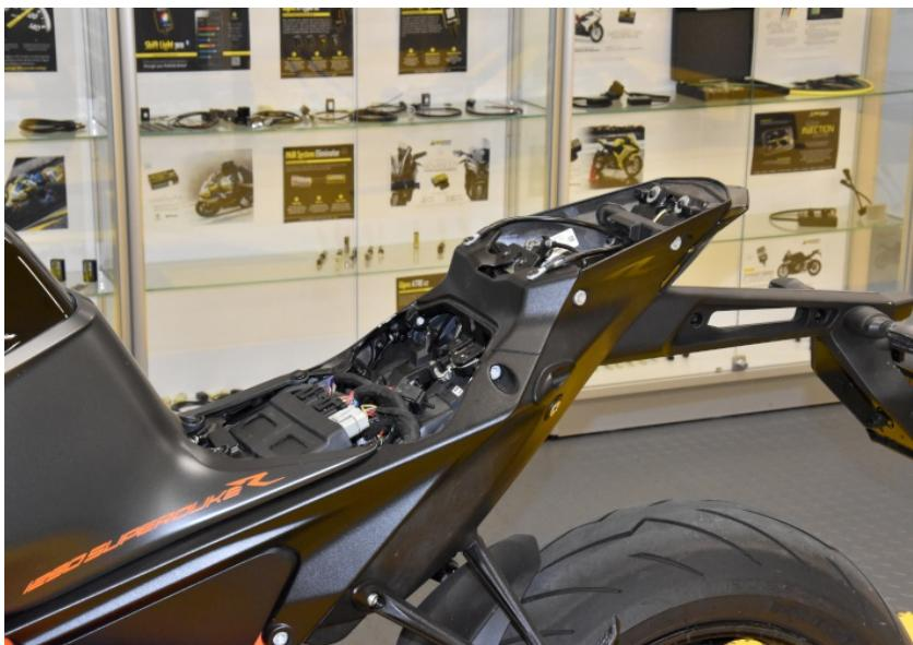
Locate the exhaust servo motor.
